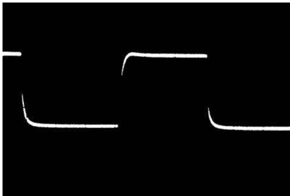
Figure 30.12(h): Loss of HF gain.
