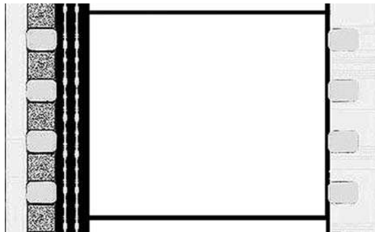
Figure 19.3: Dolby Digital as originally coded on film stock.
