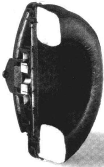
Figure 25.4: Cut-away view of a Sennheiser headphone earpiece showing the diaphragm, magnets, and acoustic damping materials.
