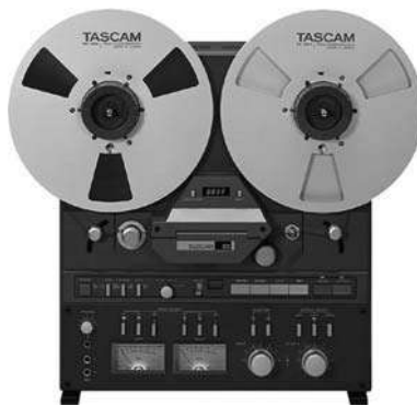
Figure 26.8: Analogue mastering recorder.
